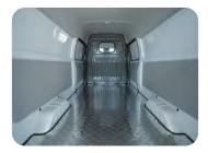
One-piece steel barrier ALL FLAT High-strength aluminum flooring designed
